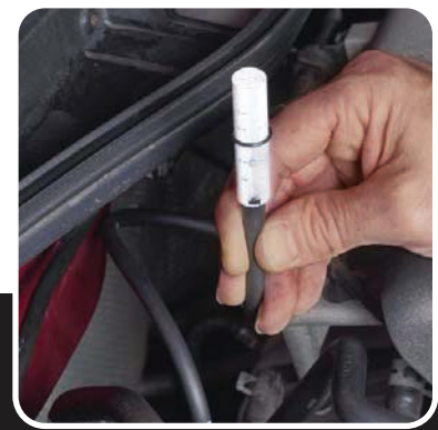
Flow meter quickly indicates presence of sealant
